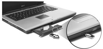
When the power is off, you can eject the drive tray using the emergency eject hole. See page 48.
